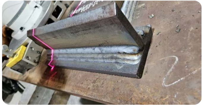
20mm Weld leg height (Accumulate welding procedure database for fillet welds with different thicknesses and processes)
