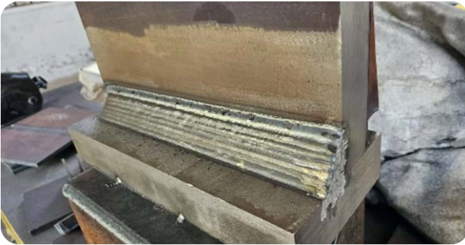
50mm Height of weld leg
